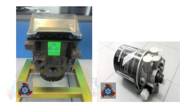
2) Every item brought in for remanufacture (sometimes referred as item reconditioning) undergoes an initial inspection and is graded before being carefully dismantled for cleaning and degreasing. Piston, seal rings and other small item are discarded as a matter of policy
