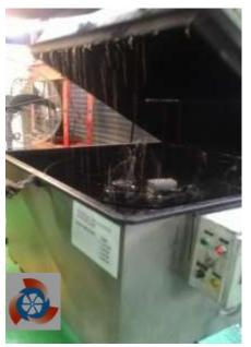
Oven Machine – To remove all dirt and rust attached to the turbine at very high temperatures to 750 Celsius.
